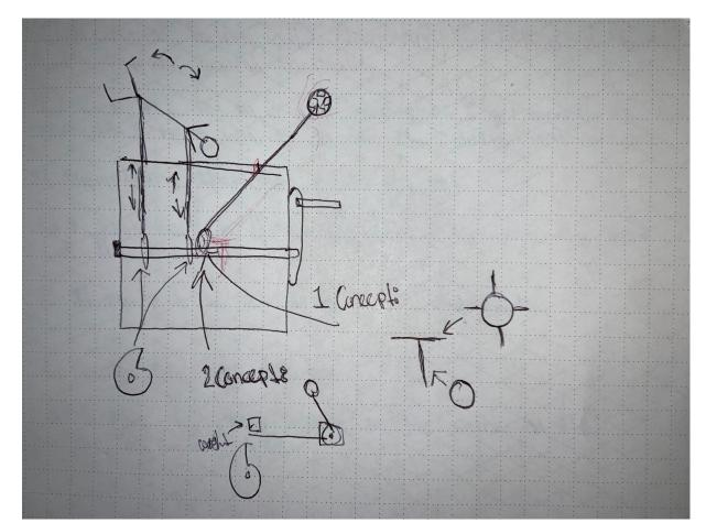
concept sketch. I had already thought about all the pieces I would have needed and how I wanted it to look. Although there was a small piece I still had not figured out, I knew the cams that I would have needed and the measurements. When it came to the ball, it wasn't as simple as I thought it would've been in my head. Getting a lever to move the opposite way of the axle and cam was a very difficult challenge.
