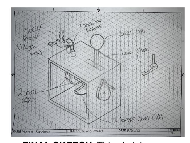
FINAL SKETCH: This sketch was made from the isometric view of the real life box using perspective and horizontal lines.
