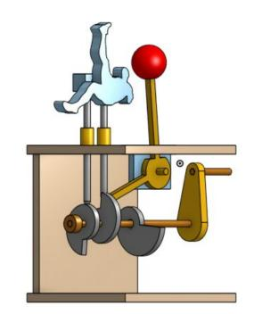
**MECHANISM VIEW:** The mechanics. The part of the project I am most proud of. Here we see how in the end after all the mates, tangent mates, and rotations, we are shown how the followers and lever line up almost perfectly to the cams. The dimensions, space, and position of each and every single cam was done purposely to get everything to move the way it was supposed to.
